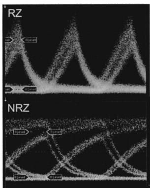
FIG. 5. RZ and NRZ eye diagrams at 2.5 Gbit/s.
