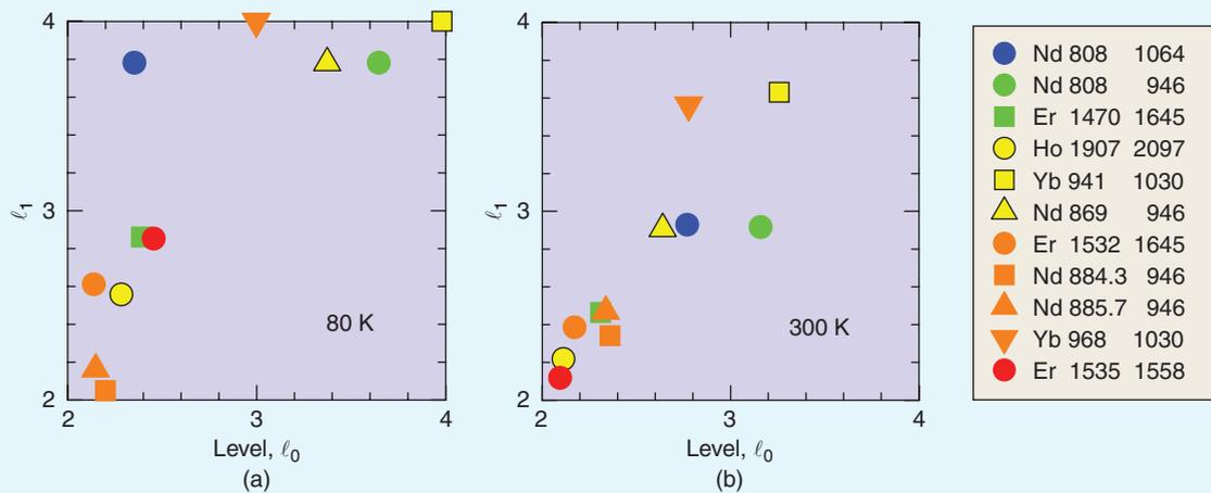
Figure 7.  $\ell_1$  vs  $\ell_0$  for a variety of known lasers at (a) 80 K and (b) 300 K. The color is keyed to the quantum defect. The best material is YAG in all cases, except in the last case, where the best is  $\text{Sc}_2\text{O}_3$ .
