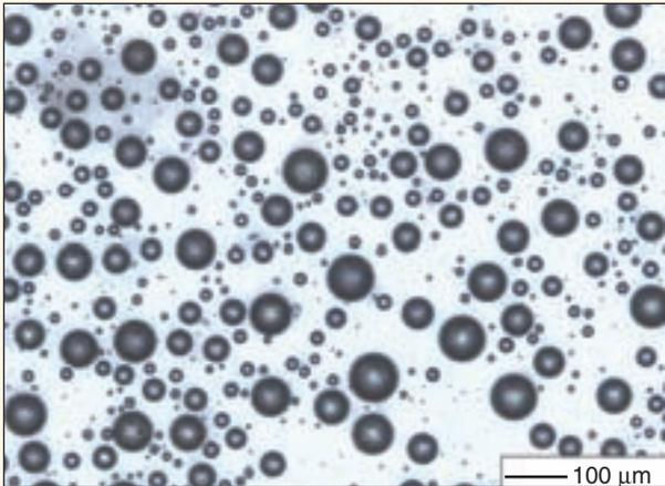
Figure 3. Optical spectroscopy experiments performed on water microdroplets that are standing on a superhydrophobic surface at Koç University (Courtesy: A. Kiraz Lab).
