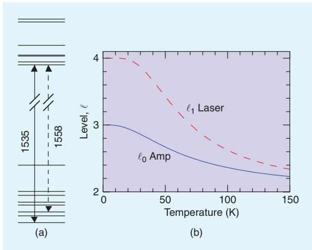
Figure 4. Er:Sc<sub>2</sub>O<sub>3</sub>,  $\lambda_p = 1535$  nm,  $\lambda_L = 1558$  nm: (a) energy levels, pump and laser transitions, (b) temperature dependence of the level parameters.
