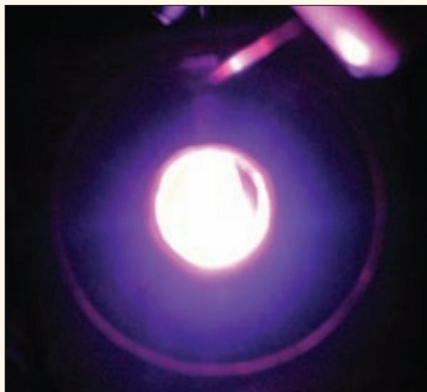
Figure 1. Exemplary white LED integrated with semiconductor nanocrystals for high-quality solid state lighting developed at Bilkent University (Courtesy: H. V. Demir Lab).
