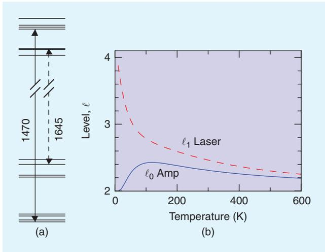
Figure 3. Er:YAG,  $\lambda_p = 1470$  nm,  $\lambda_L = 1645$  nm: (a) energy levels, pump transition (solid line), and laser transition (dashed line), (b) temperature dependence of the level parameters.
