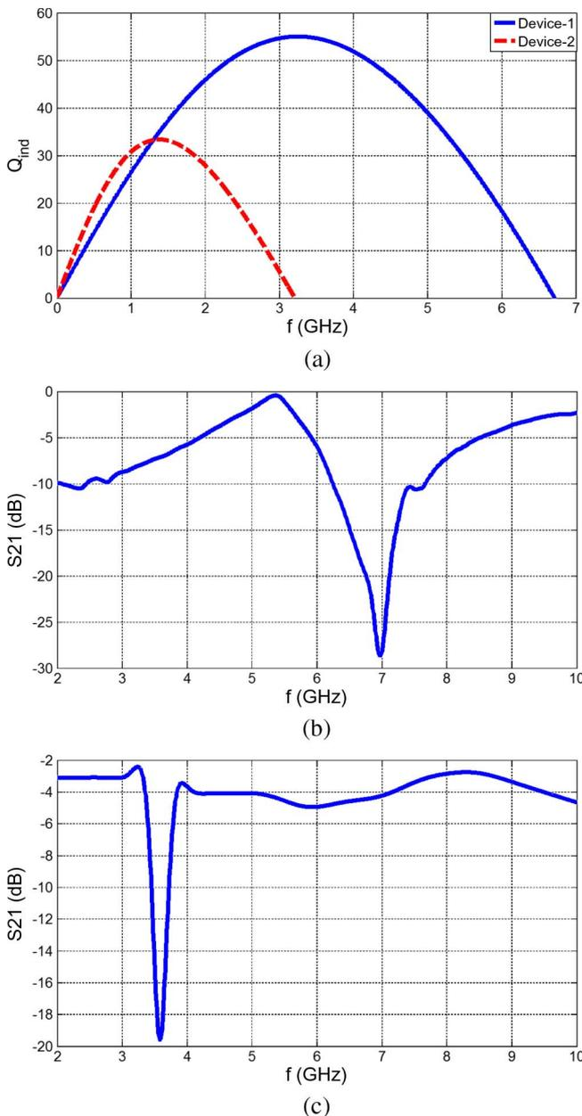
Fig. 10. (a)  $Q_{ind}$  of Device-1 and Device-2. (b) Experimental  $S_{21}$  parameter of Device-1 with respect to frequency. (c) Experimental  $S_{21}$  parameter of Device-2 with respect to frequency.
