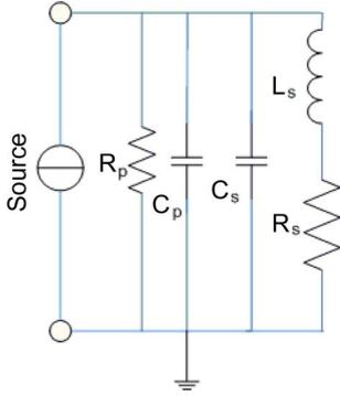
Fig. 2. Conventional simplified one-port parallel RLC circuit.
