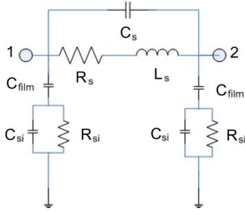
Fig. 1. Conventional lumped-element circuit model.
