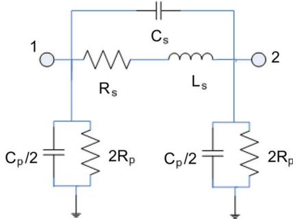
Fig. 3. Our two-port circuit model to calculate the  $Q$ -factor.
