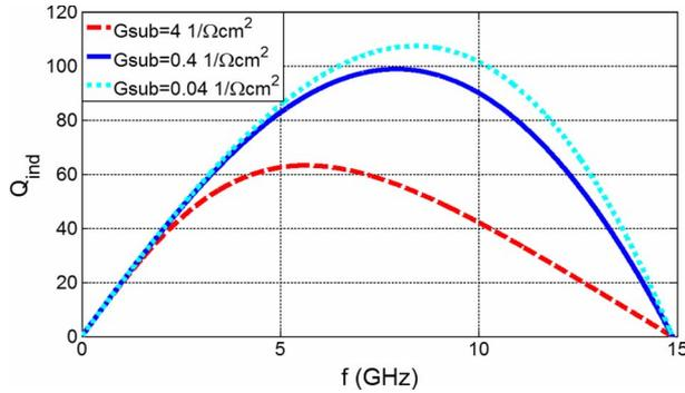
Fig. 4. Relationship between  $Q_{\text{ind}}$  and substrate resistivity.
