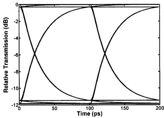
FIG. 5. Simulation of 10 Gb/s nonreturn-to-zero operation (for a 2- $\mu\text{m}$ -wide  $\times$  250- $\mu\text{m}$ -long, center bias point device using an average incident control power of 4.65 mW at  $\lambda_{\text{control}}=822$  nm and  $\lambda_{\text{signal}}=864$  nm with  $R_{\ell}=16$   $\Omega/\mu\text{m}$  and  $C_{\ell}=0.23$  fF/ $\mu\text{m}$ ).
