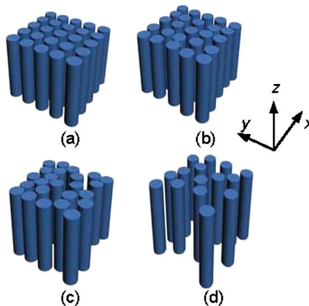
Fig. 1. (Color online) Schematics of silicon NW arrays with (a) regularly arranged square lattice, (b) random NW contained in regular unit cell used in [20], (c) 48% position random, and (d) 30% position random structure.
