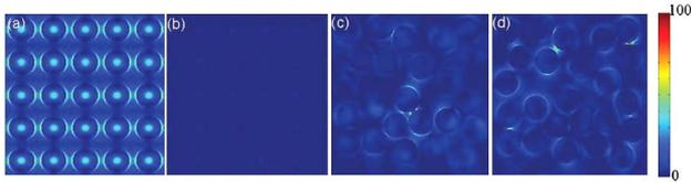
Fig. 3. (Color online)  $E$ -field distributions in a regularly arranged NW array at (a)  $\lambda = 899.1$  nm and (b)  $\lambda = 916.0$  nm.  $E$ -field distributions in a 48% position random NW array at (c)  $\lambda = 899.1$  nm and (d)  $\lambda = 916.0$  nm.
