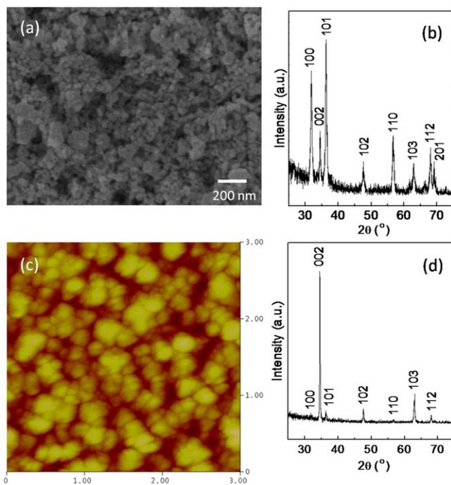
**Figure 1.** SEM image of ZnO porous film fabricated on Ti substrate (a) and its XRD pattern (b). AFM images of the GZO counter electrode deposited on glass substrate by MOCVD (the unit of scale bar is  $\mu\text{m}$ .) (c) and its XRD pattern (d).
