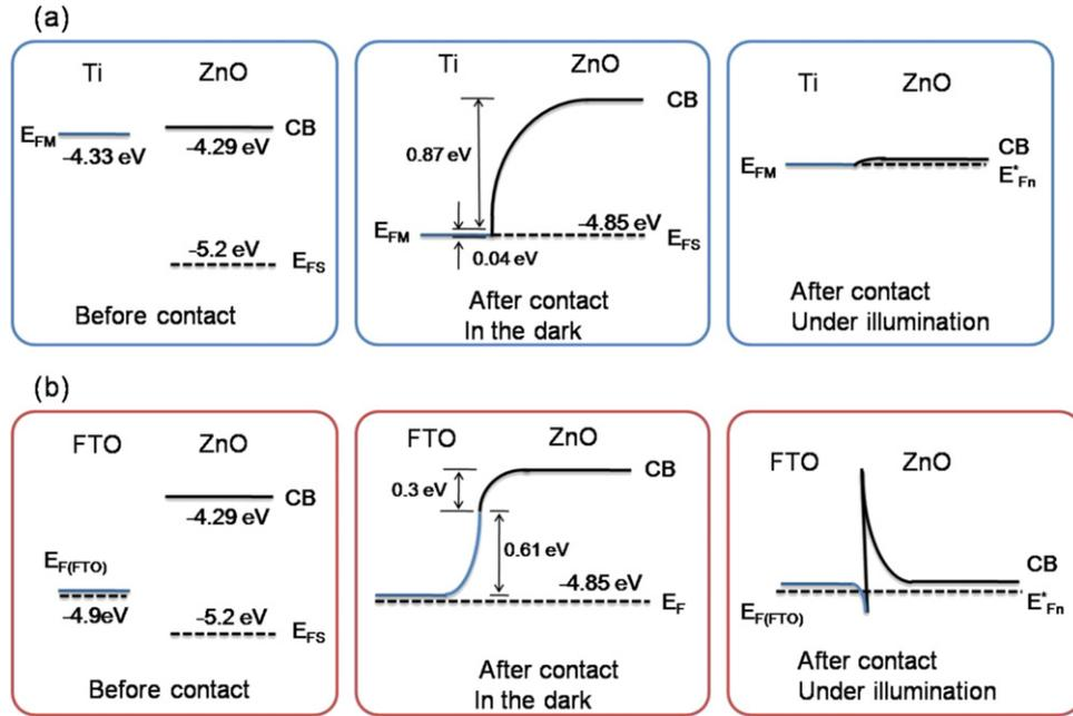
**Figure 6.** Schemes of electron energy at (a) Ti/ZnO contact and (b) FTO/ZnO contact. Left diagrams illustrate the energy level of individual layers before contact, centre ones show the band bending at the interface in the dark, and right diagrams show the formation of ohmic and Schottky contact for Ti/ZnO and FTO/ZnO, respectively, under strong illumination and open circuit conditions.
